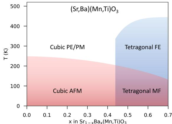
FIG. 1. Phase diagram for  $\text{Sr}_{1-x}\text{Ba}_x\text{Mn}_{1-y}\text{Ti}_y\text{O}_3$  as a function of temperature and barium content  $x$ . Compositions with  $x \geq 0.5$  are synthesized with dilute amounts of Ti on the Mn site. Compiled from results published in Refs. 8, 11, and 12. PE = paraelectric; PM = paramagnetic; FE = ferroelectric; AFM = antiferromagnetic; MF = multiferroic.
