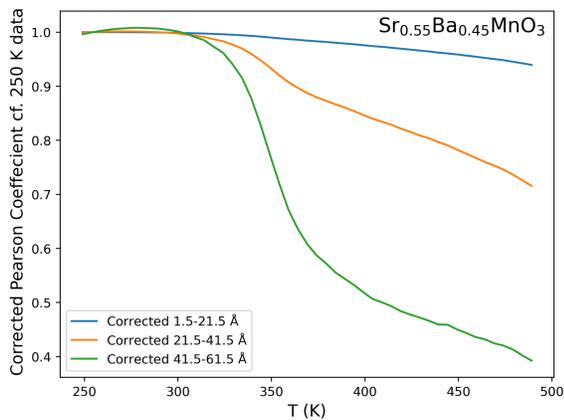
FIG. 5. Pearson correlation coefficient for  $\text{Sr}_{0.55}\text{Ba}_{0.45}\text{MnO}_3$  with respect to the x-ray PDF data collected at 250 K, corrected for thermal expansion as explained in the main text. Three different data ranges are used. The ferroelectric transition around 350 K is most evident for the highest  $r$ -range but essentially invisible for the shortest data range, confirming that the local structure is already symmetry broken above  $T_C$ .
