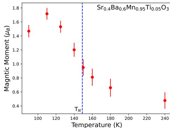
FIG. 9. Locally ordered magnetic moment in  $\text{Sr}_{0.4}\text{Ba}_{0.6}\text{Mn}_{0.95}\text{Ti}_{0.05}\text{O}_3$  obtained from mPDF analysis. The persistent ordered moment above  $T_N$  arises from short-range AFM correlations. The anomalous drop in the ordered moment at 90 K is expected to be an artifact of imperfect thermal equilibrium.
