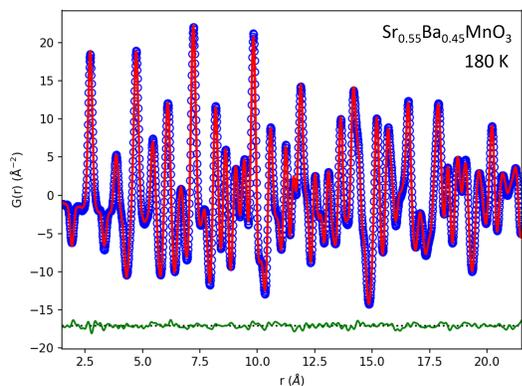
FIG. 6. Representative neutron PDF fit for  $\text{Sr}_{0.55}\text{Ba}_{0.45}\text{MnO}_3$  at 180 K. The blue symbols show the experimental data, the red curve the best fit, and the green curve the fit residual, offset vertically for clarity.
