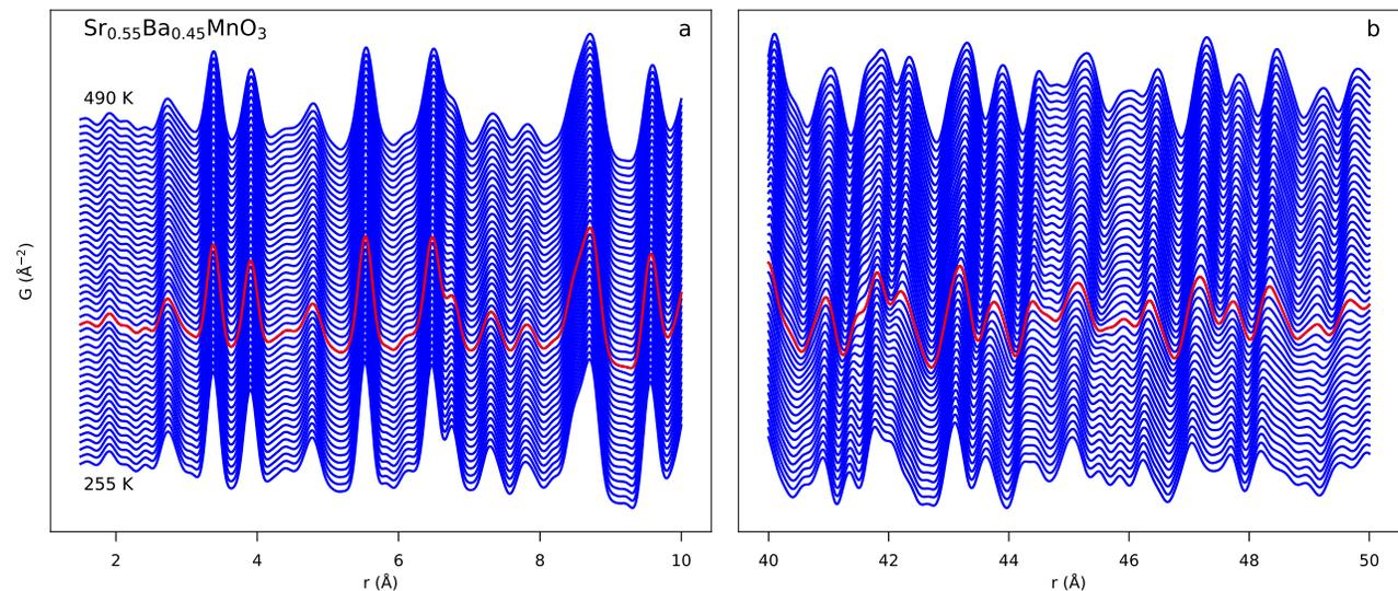
FIG. 3. X-ray PDF data for  $\text{Sr}_{0.55}\text{Ba}_{0.45}\text{MnO}_3$  between 250 K and 490 K displayed over the range 1.5 – 10 Å (a) and 40 – 50 Å (b). The PDF patterns were collected in increments of 5 K and are offset vertically on the plot for clarity. For the viewing range at higher  $r$ , clear and abrupt changes are evident across the ferroelectric transition at 350 K (red PDF pattern). No abrupt changes are observed in the low- $r$  viewing range.
