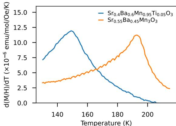
FIG. 2. Temperature derivative of the magnetic susceptibility of  $\text{Sr}_{0.4}\text{Ba}_{0.6}\text{Mn}_{0.95}\text{Ti}_{0.05}\text{O}_3$  and  $\text{Sr}_{0.55}\text{Ba}_{0.45}\text{MnO}_3$  as a function of temperature. Maxima occur at 149 K and 193 K, respectively. The measurements were taken in a field of 1 T using a zero-field-cooling protocol.
