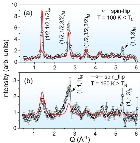
FIG. 10. Spin-flip magnetic scattering from  $\text{Sr}_{0.4}\text{Ba}_{0.6}\text{Mn}_{0.95}\text{Ti}_{0.05}\text{O}_3$  at 100 K [(a); AFM state] and 160 K [(b); PM state]. The black symbols show the experimental data, while the red curves are calculated based on the model explained in the main text. Nuclear Bragg peaks causing artifacts in the magnetic signal are indicated with a subscript N.
