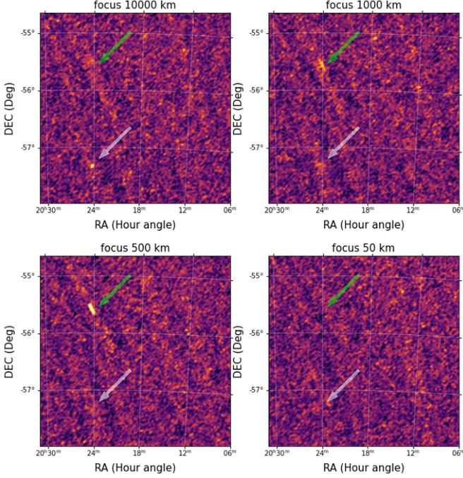
**Figure 2.** MWA images for four different focal distances. In all four panels, the green arrows show the location of the ISS signal and the white arrow shows the location of a background astronomical point source. We note that at large focal distances, the objects in the near-field (e.g ISS) appear de-correlated and at much closer focal distances the background far-field sources appear de-correlated. An animation of this Figure is available at <https://www.youtube.com/watch?v=sqiejYJCAo>.
