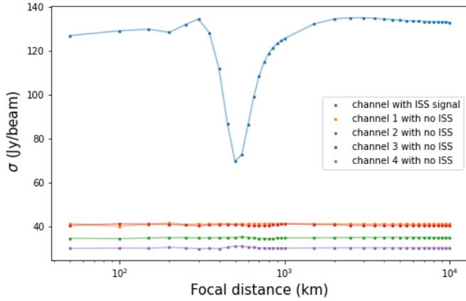
**Figure 6.** Noise levels in residual maps for five different channels focused to a wide range of focal distances. Note that the noise is lowest in the channel with the ISS when the focal distance is approx. 500 km (also the line of sight range to ISS)
