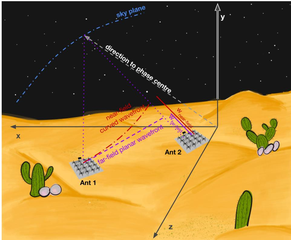
Figure 1. The Topocentric Cartesian Coordinate (TCC) system used in this work to calculate near-field corrections.
