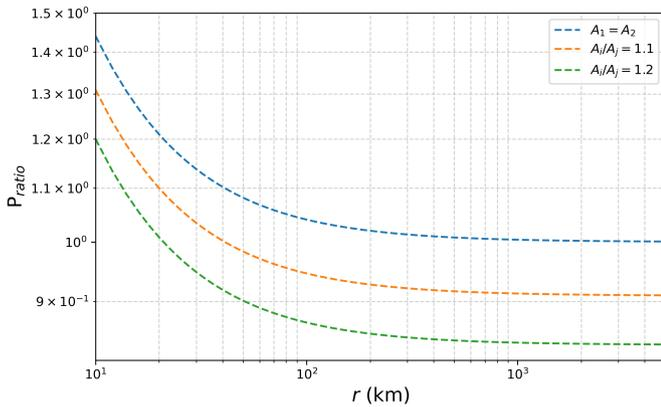
**Figure 5. updated figure** We show the ratio of powers seen by a baseline with ( $A_1$  not equal to  $A_2$ ) and without ( $A_1 = A_2$ ) holographic effects. For the above plot, we assume  $\Delta r = 2$  km (approx. delay in a 6 km baseline observing a source 20 degrees from the zenith).
