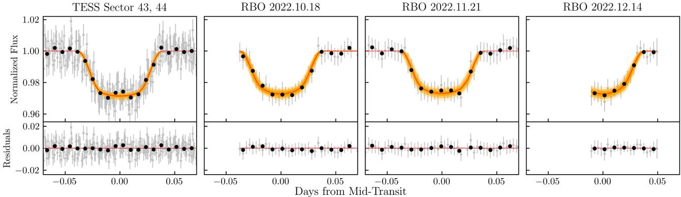
**Figure 2.** The raw (grey) and 10-minute-binned (black) phase-folded light curves of TESS and RBO photometry. The best joint fit model is shown in red, and the  $1\sigma$ ,  $2\sigma$ , and  $3\sigma$  confidence intervals are shown in yellow with descending intensities.
