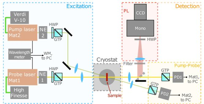
FIG. 1. Scheme of the experimental setup: Two tunable dye laser are used to excite the sample. Both lasers beams are detected by photodiodes. Photoluminescence is detected by a combination of monochromator and CCD camera. Abbreviations: WM: wavelength meter; NE: noise eater; HWP: half-wave plate; GTP: glan-taylor prism; PD: photodiode; Mat1/2: Matisse 1, Matisse 2; CCD: charge-coupled device camera.
