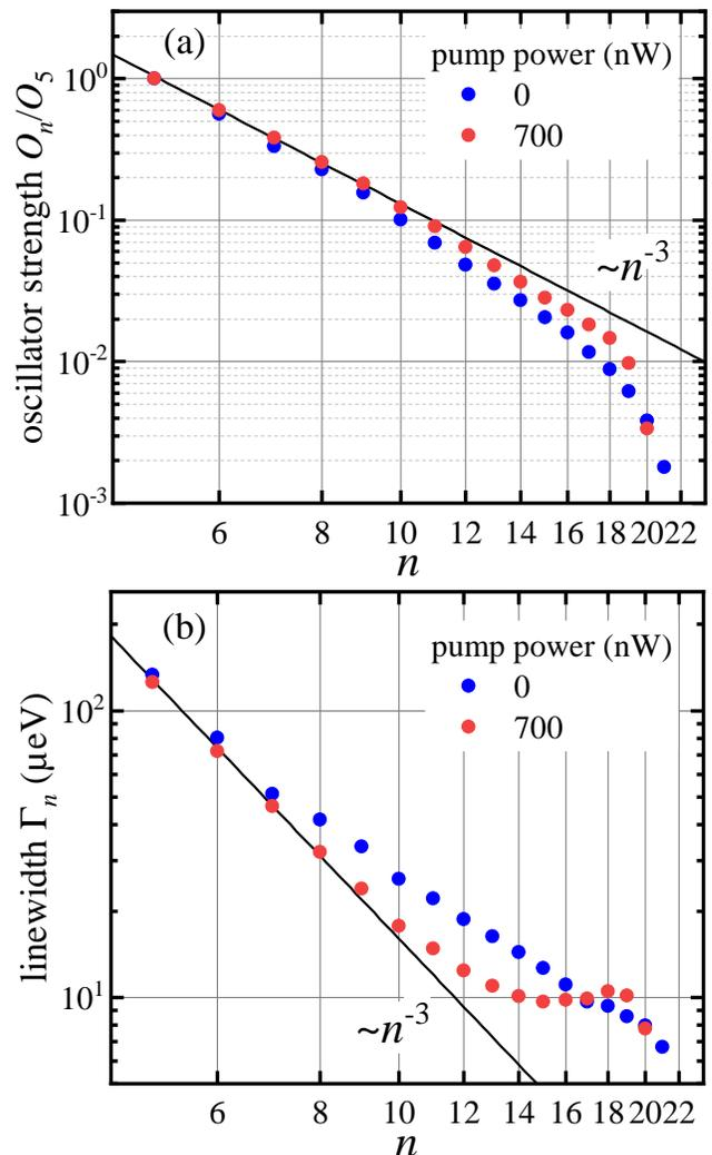
FIG. 3. Normalized oscillator strengths (a) and linewidths (b) from the spectra in Fig. 2 at zero pump power (blue) and at 700 nW (red) obtained by fits according to Eq. (1). In both panels the black solid lines shows the expected dependence following  $n^{-3}$ .
