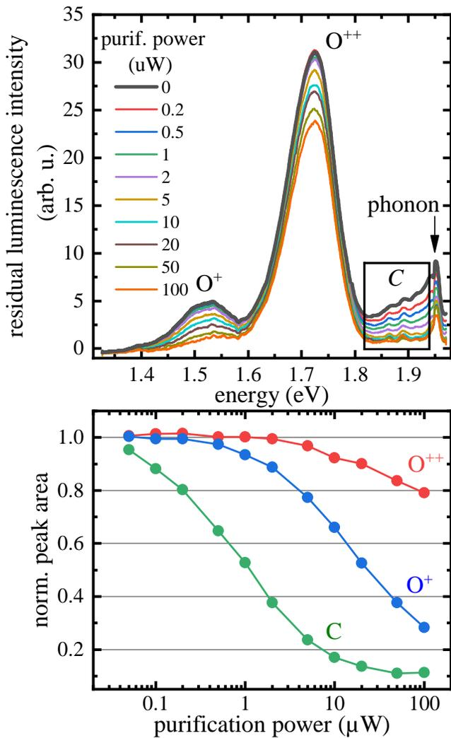
FIG. 9. Residual PL intensity of defects in sample I under above-band-gap excitation at 2.033 eV and additional *purification* laser excitation at  $\tilde{E}_g$  with varying powers. Both  $O^+$ ,  $O^{++}$  as well as the signal in range **C** decrease with increasing power of the additional laser. (b) Peak areas from the signals in panel (a) obtained by a fit (see text) normalized to the value in the absence of additional laser excitation.
