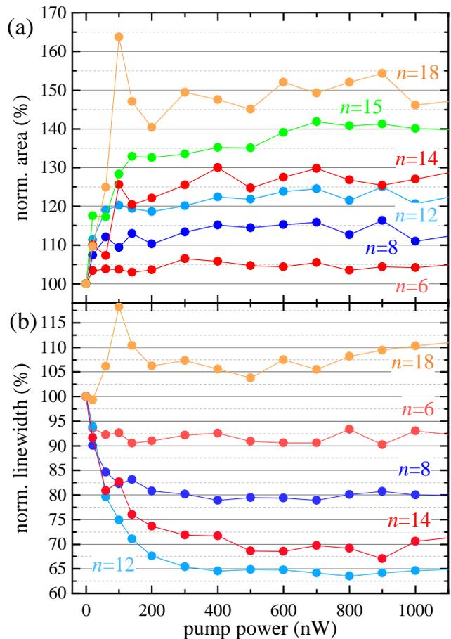
FIG. 5. Analysis of (a) oscillator strengths  $O_n$  and (b) linewidths  $\Gamma_n$  as a function of pump power for even principal quantum numbers measured at a probe power of 200 nW. The pump laser energy is set to  $\tilde{E}_g$ . The pump power range is restricted to the pump power range of purification, i.e. below 2  $\mu\text{W}$ . The values are normalized to the corresponding value at zero pump power to visualize the change in percent.
