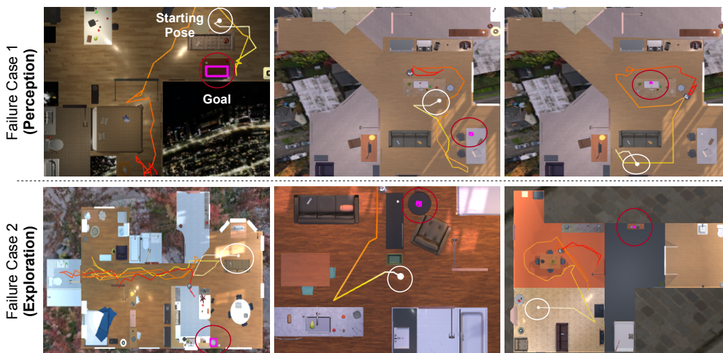
Figure 9: Failure cases of EmbCLIP-Codebook in Object Navigation. Top row shows the failure examples related to perception, where the agent traverses past the goal object but fails to identify it. The bottom row shows another failure mode where the agent fails to explore specific areas of the environment where the target object is located. (Agent’s starting pose is shown in white circle and the target object is shown in a red circle)
