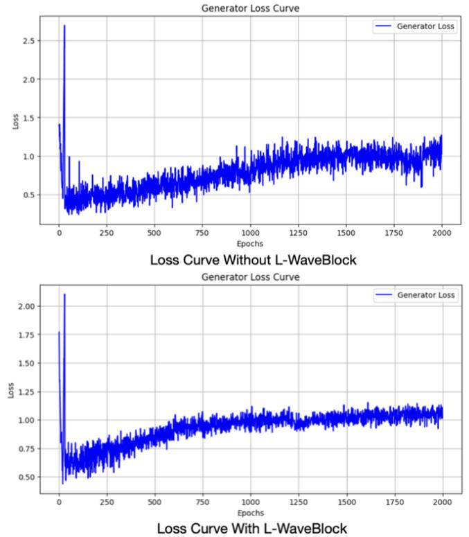
Fig. 8. Loss curve with and without L-WaveBlock for maps imagery dataset
