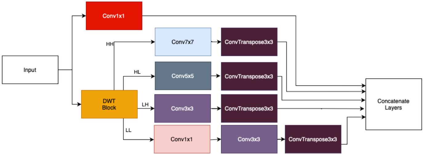
Fig. 2. L-WaveBlock Architecture
