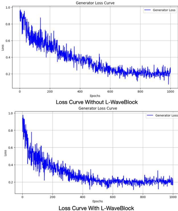
Fig. 10. Loss curve with and without L-WaveBlock for SRGAN dataset
