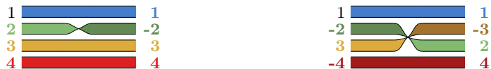
(a) The 1-twist changes 1\ 2\ 3\ 4 into 1\ \bar{2}\ 3\ 4 . (b) The 2-twist changes 1\ \bar{2}\ 3\ \bar{4} into 1\ \bar{3}\ \bar{2}\ \bar{4} .
