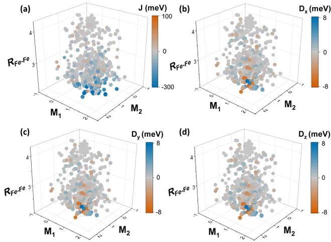
**Figure 3.** Magnetic exchange couplings ( $J$ ) and three components of the DMI vectors are shown as 3D scatter plots and with heat-map depending on their strengths. The x and y axes show the magnetic moments ( $\mu_B$ ) of the Fe ions from the pairs. The z-axis is the distance ( $\text{\AA}$ ) between the Fe pairs.
