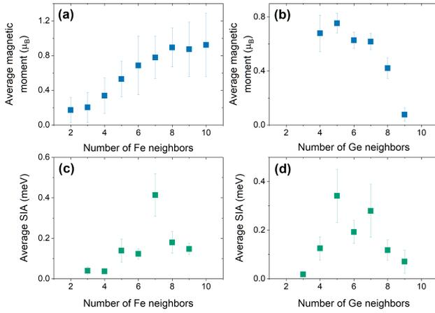
**Figure 2.** (a,b) The average magnetic moment and (c,d) SIA as a function of the number of Fe and Ge neighbors within  $3.5\text{\AA}$ . Error bars are the standard deviation in the magnetic moments with respect to the average magnetic moment of Fe ions.
