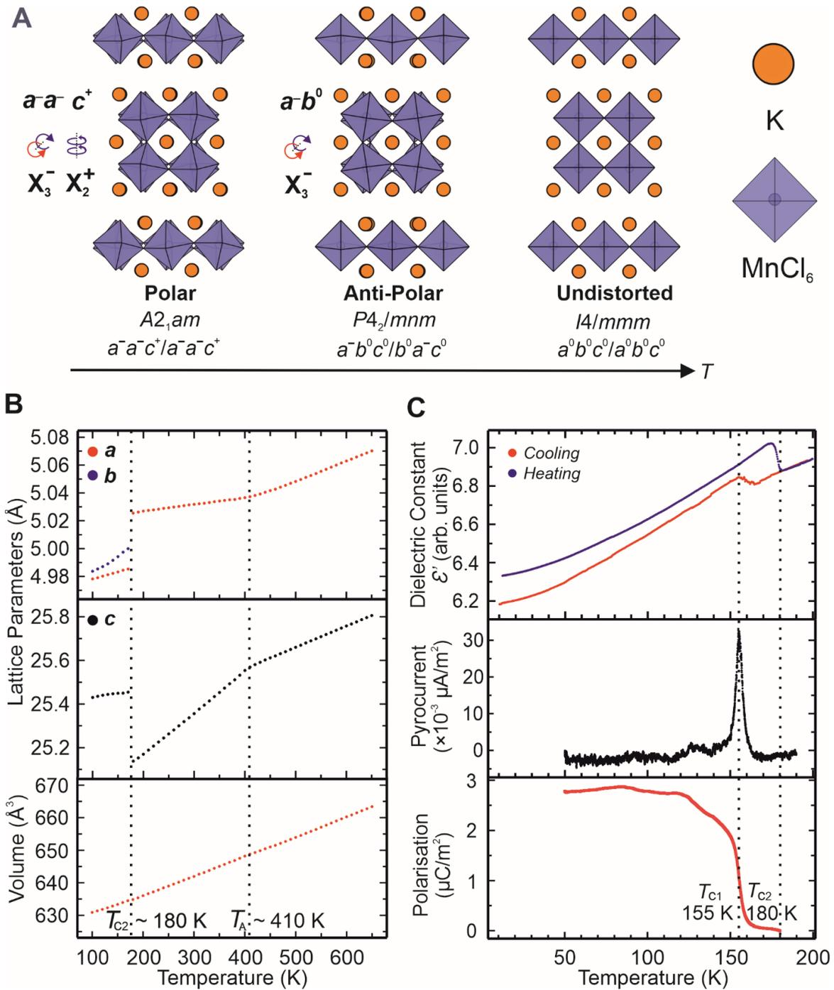
**Fig. 1. Structure evolution of  $K_3Mn_2Cl_7$ .** (A) Schematic of tilting distortions adopted by  $K_3Mn_2Cl_7$  with temperature. (B) Normalized lattice parameters with temperature. (C) Temperature-dependent dielectric constants, pyroelectric currents and electric polarizations on a polycrystalline pellet.
