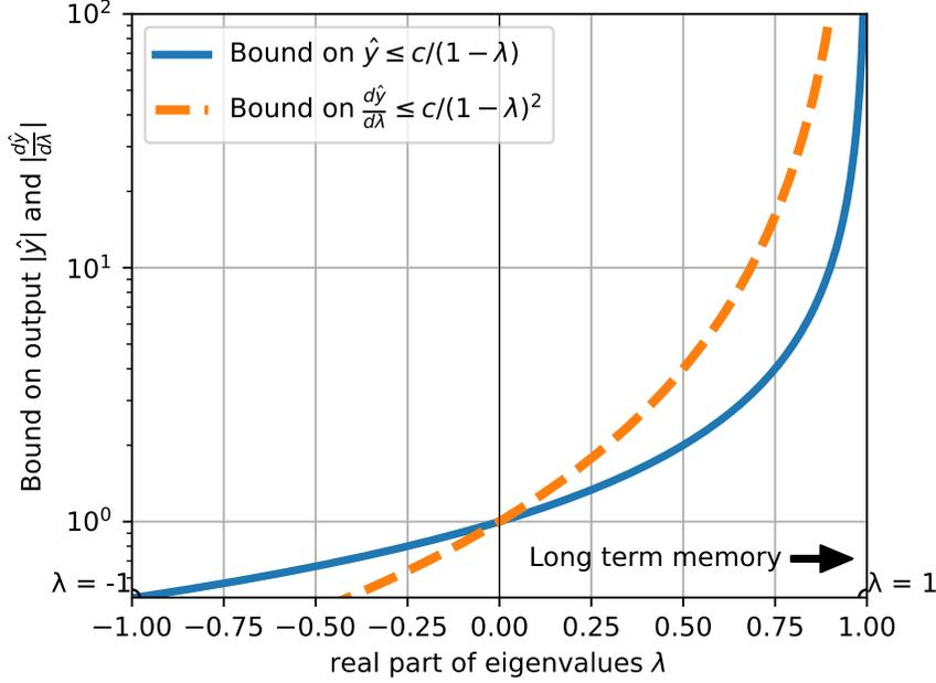
Figure 2. The scaling of layer output bound  $|\hat{y}| \leq \frac{c}{1-\lambda}$  and the gradients  $|\frac{d\hat{y}}{d\lambda}| \leq \frac{c}{(1-\lambda)^2}$ . The stability boundary is  $\lambda = \pm 1$ . When the model adapts to learn long-term memory (as  $\lambda$  approaches 1), the gradient experiences an increase that surpasses the rate of output growth. Techniques like layer normalization are insufficient to address this issue of exploding gradients effectively.
