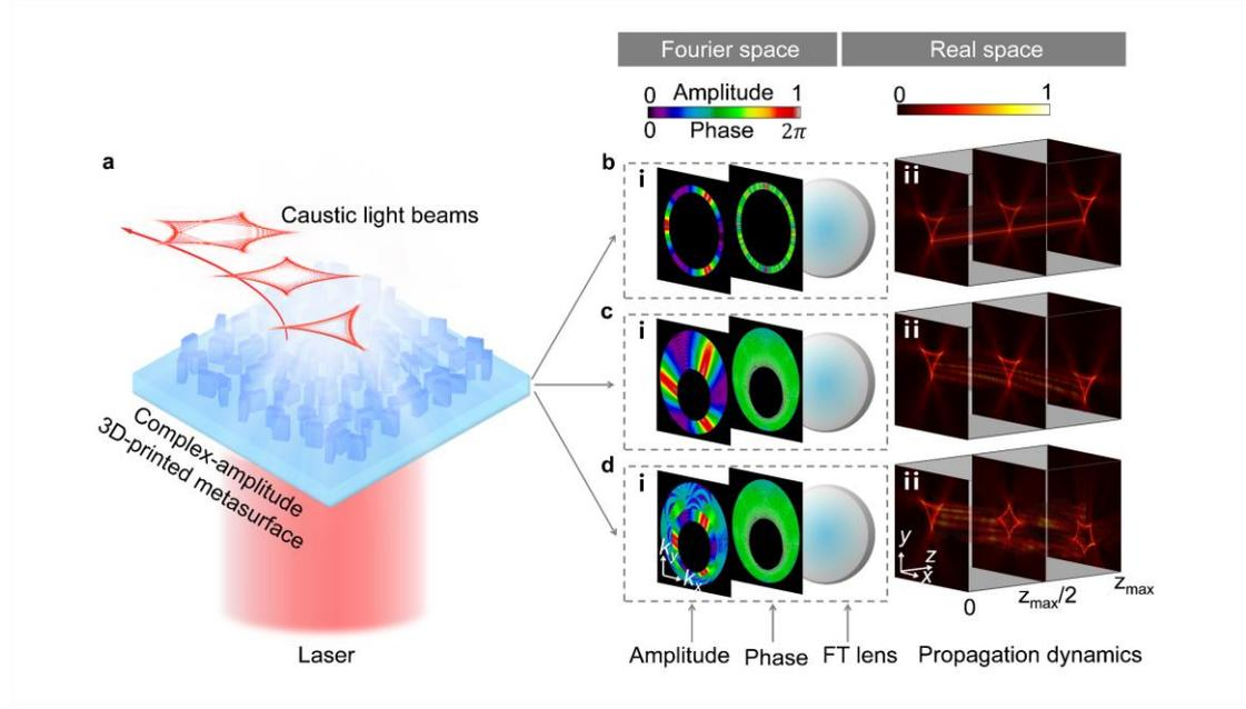
**Fig. 1 Principle of arbitrary engineering of spatial caustics based on 3D-printed metasurfaces.** **a** Schematic of customized optical caustics, generated by the metasurface. **b(i)-d(i)** Amplitude and phase information of the desired caustic beams in Fourier space, together with a FT lens. **b(ii)-d(ii)** Propagation dynamics of realized caustic structured light in real space.
