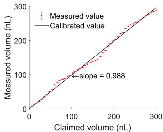
**Fig. S6 Calibration of dispensed liquid volume.** A series of liquid volumes claimed by the dispenser was dispensed on the glass substrate to form the liquid lens, and the volume was measured (with a measurement accuracy of  $\pm 0.05$  nL). The slope of the fitted line is about 0.988 and is used to calibrate the claimed dispensed volume.
