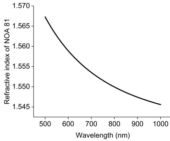
**Fig. S7 Refractive index profile of NOA 81 under room temperature.**
