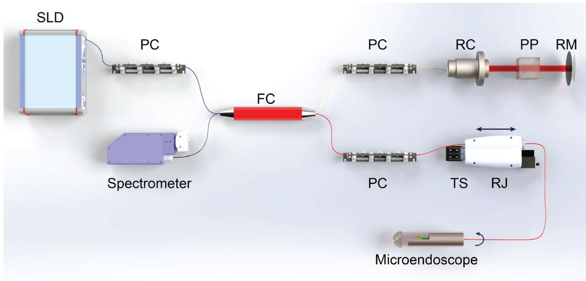
**Fig. S3 Schematic of the endoscopic spectral-domain OCT (SD-OCT) system working near 800 nm.** SLD: superluminescent diode, PC: polarization controller, FC: fiber coupler, RC: reflective collimator, PP: prism pairs, RM: reflective mirror, TS: translational stage, RJ: rotary joint.
