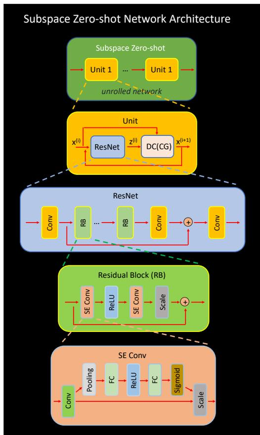
Figure 2: Network structure of each sub-network. We introduce SE convolution which is a kind of attention mechanism based on ZSSSSub method.
