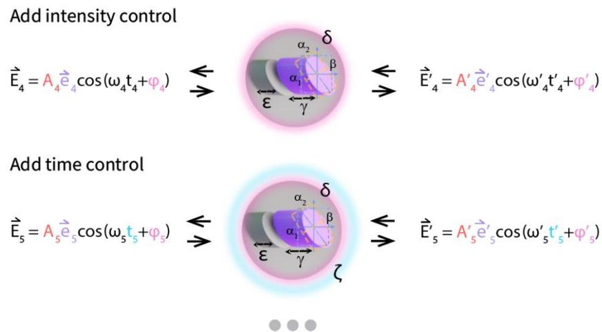
Fig. 6: **Extended functionalities of the synthetic matter approach.** By adding more devices, the matter would be able to manipulate the intensity values as well as the degrees of polarisation (through time control), as well as enriching its own vectorial properties. The  $\epsilon$  and  $\zeta$  in the figure present attenuation value and depolarisation value. The manipulation mechanism and further discussion can be found in Methods 6, 7, 8 and extended Figure 8.
