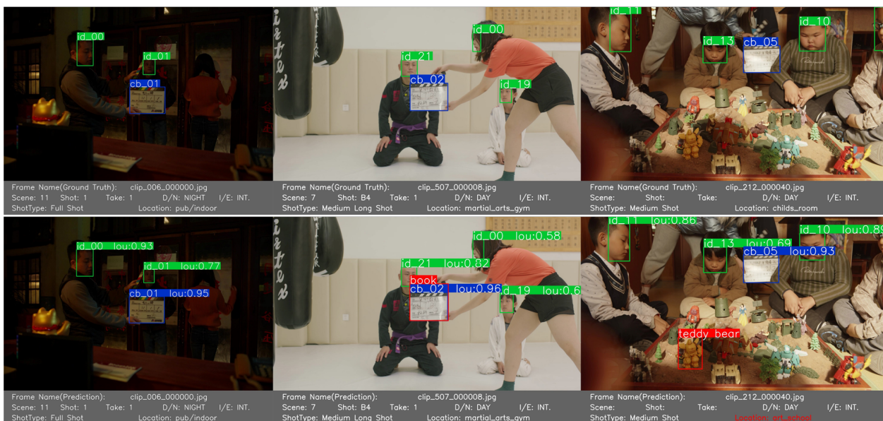
Figure 5: Region predictions and semantic annotations in Film-RVSAD. We use our method to generate metadata for video search and retrieval. Examples in the upper line are ground-truths in Film-RVSAD, and examples in the bottom line are results from our proposed system.
