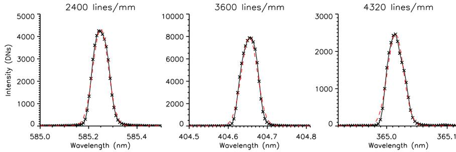
**Figure 11.** The solid black lines are example spectral profiles captured by the same fibre core for the 585.249 nm (left panel), 404.656 nm (middle panel), and 365.016 nm (right panel) calibration lamp emission lines using the 2400 lines/mm, 3600 lines/mm, and 4320 lines/mm diffraction gratings, respectively. The dashed red lines denote the fitted Gaussian for each emission profile, which determines the associated FWHM for that feature.
