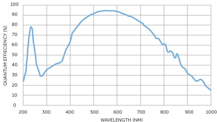
**Figure 4.** The quantum efficiencies (QEs) of the *Princeton Instruments* Kuro 2048B scientific CMOS camera chosen to image the fibre-resolved spectra. FRANCIS operates within the wavelength range of 390 – 700 nm, hence this camera provides QEs > 60 % across the useable wavelength domain. This image is kindly reproduced from the Teledyne Imaging Group resource centre (<https://www.photometrics.com/learn/imaging-topics/quantum-efficiency>).
