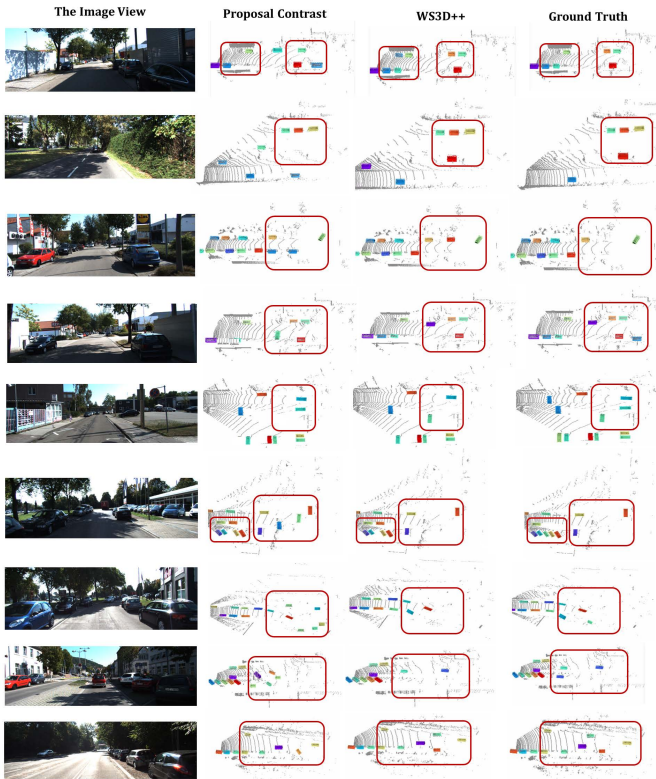
Fig. 8: The object detection comparisons on KITTI [128] validation set. It can be demonstrated that our proposed WS3D++ provides very accurate bounding box predictions qualitatively compared with the previous state-of-the-art merely using 2D bounding boxes, which demonstrates the effectiveness of using 3D regional as well as 3D object-level information in facilitating effective feature representation learning.
