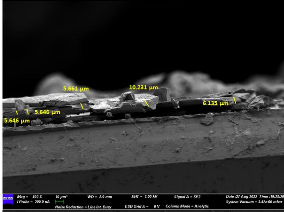
**Figure S8.** SEM image of the Cs<sub>3</sub>Sb<sub>2</sub>Cl<sub>9</sub> crystallites showing an average thickness of 6.91 μm.
