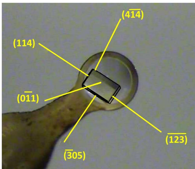
**Figure S1.** SCXRD measurement on top of the planar surface of a single crystal revealing (114) lattice planes perpendicular the elongated surface of the rod.
