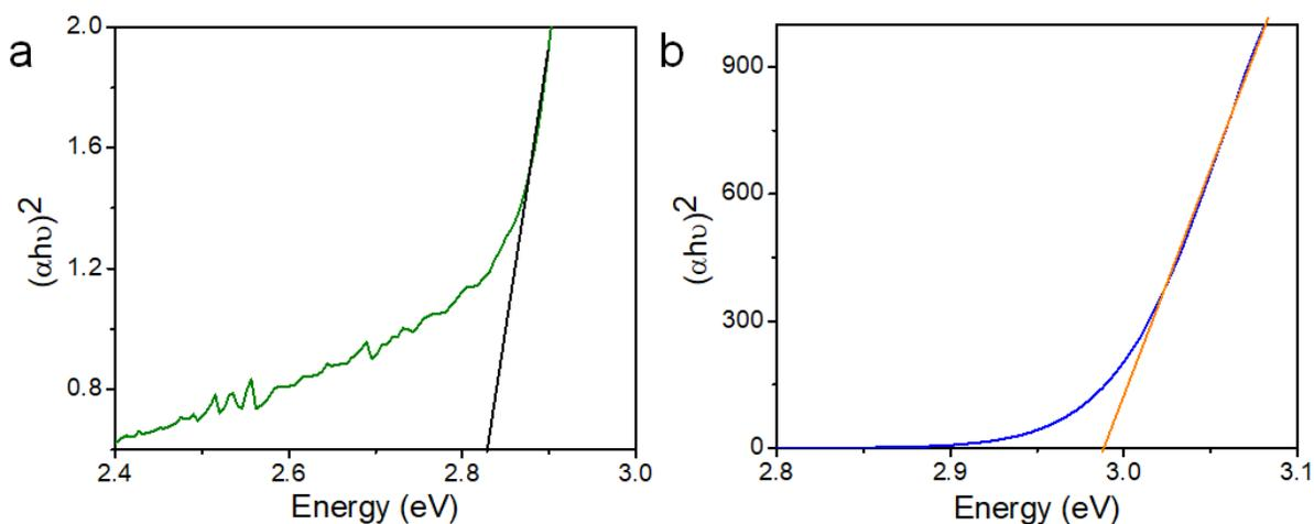
**Figure S7.** Tauc plot from (a) UV-Visible Spectroscopy showing the band gap of 2.86 eV (b) Diffuse Reflectance Spectroscopy, showing the band gap of 2.98 eV of the Cs<sub>3</sub>Sb<sub>2</sub>Cl<sub>9</sub> single crystals.
