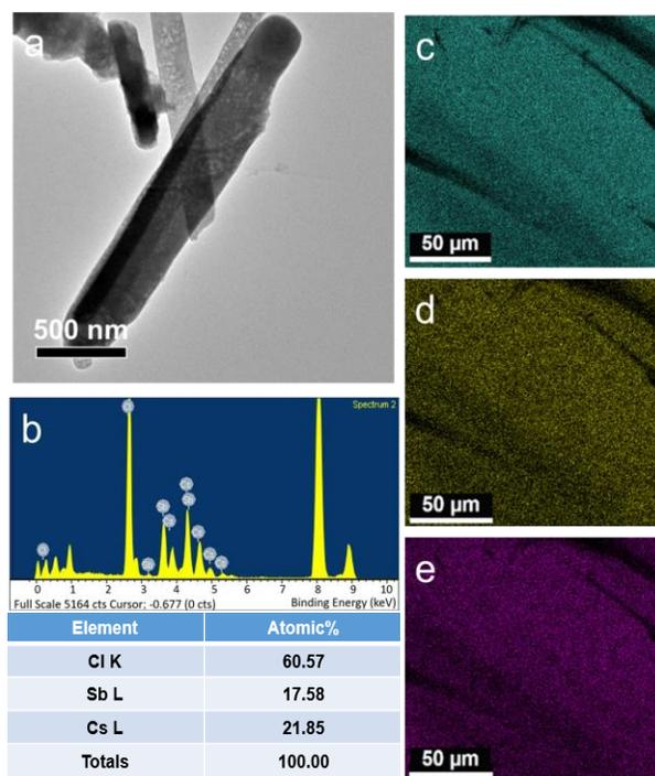
**Figure S4.** TEM analyses of finely grinded  $\text{Cs}_3\text{Sb}_2\text{Cl}_9$  single crystals. (a) TEM image. (b) EDS spectrum revealing the elemental analyses EDS spectrum shows a ratio of 3:2:7 of Cs:Sb:Cl. (c-e) HAADF-STEM image and EDS elemental mapping showing homogeneous distribution of Cs, Sb, and Cl elements.
