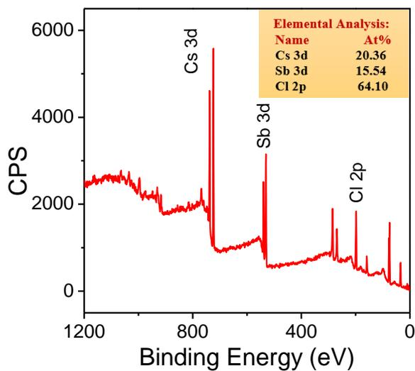
**Figure S6.** X-ray photoelectron spectroscopy survey spectrum of  $\text{Cs}_3\text{Sb}_2\text{Cl}_9$  single crystals.
