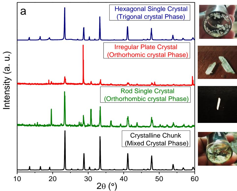
**Figure S2.** Powder XRD pattern and photographs of  $\text{Cs}_3\text{Sb}_2\text{Cl}_9$  single crystals grown from different concentrations of the precursor solution of cesium and antimony chloride in concentrated HCl, as well as under different heating condition in some cases.
