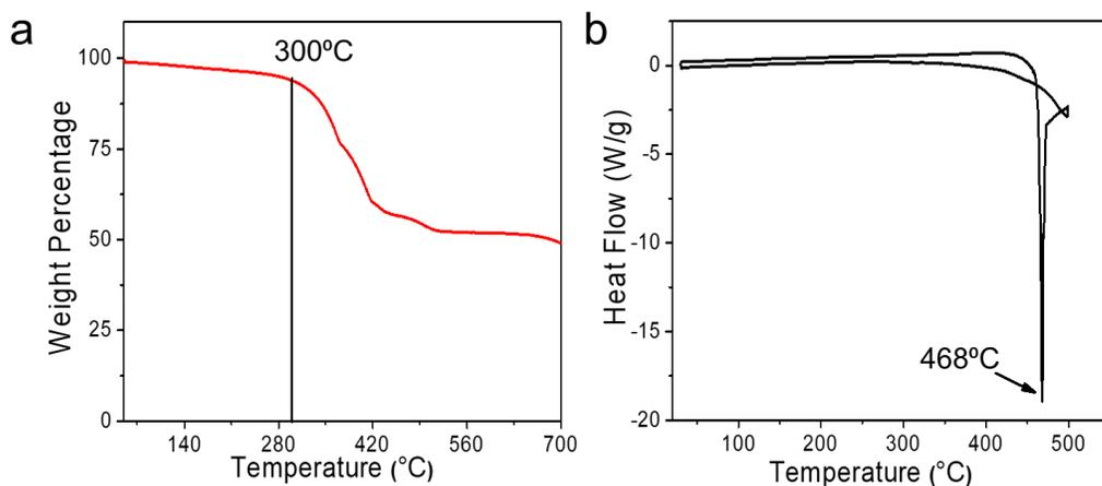
**Figure S5.** (a) Thermogravimetric analysis curve of  $\text{Cs}_3\text{Sb}_2\text{Cl}_9$  single crystals. (b) Differential scanning calorimetry curve of  $\text{Cs}_3\text{Sb}_2\text{Cl}_9$  single crystals.
