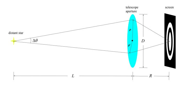
FIG. 1: Diagram showing light rays originating from a distant star passing through the telescope aperture and forming a sharp image on the screen. Here the star-aperture distance, aperture diameter, and aperture-screen distance are denoted by L, D, and R, respectively. Two distinct points on the aperture, denoted by two-dimensional vectors  $\rho$  and  $\rho'$ , span an angle of  $\Delta\theta$ . Typically  $L \gg R \gg D$ . The diagram is not drawn to scale.
