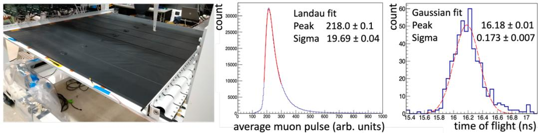
**Figure 3.** Left: bottom TOF layer, showing the 8 scintillator paddles. Middle: average integrated muon pulse signal (average of top, bore and bottom scintillators). The solid red line is a Landau fit, with a sigma/peak ratio of 9.0%. Right: distribution of time-of-flight values for near-vertical muons traversing the central regions of a top and bottom scintillator. The dashed red line is a Gaussian fit with a sigma of  $\sim 170$  ps.
