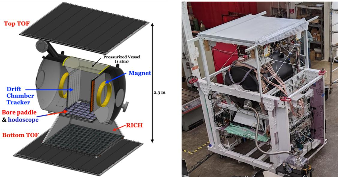
**Figure 2.** Left: a rendering of the HELIX detector arrangement. Right: the assembled HELIX instrument at a 2022 thermal-vacuum test at the NASA Neil A. Armstrong Test Facility.
