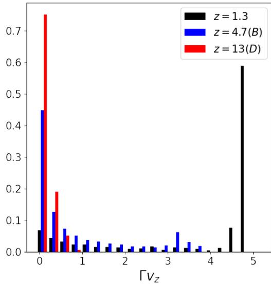
**Fig. 5.** The histogram displays the fraction of cells with a given jet velocity  $\Gamma v_z$  at the end of the simulation, calculated on three  $z = z^*$  planes, representing the initial jet, the jet after the anti-node (as in Fig. 3B) that has entrained material, and the jet further in  $z$ , where it has become sub-relativistic (as in Fig. 3D).
