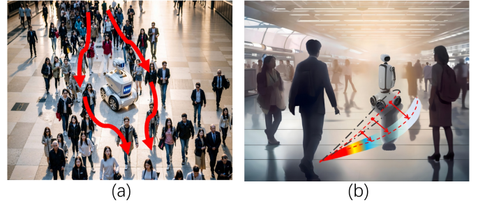
Fig. 1. Disturbance in the navigation of robots and pedestrians encompasses two key aspects. (a) At a macroscopic level, the mere presence of a robot and its trajectory can exert influence on the flux of pedestrian flow, affecting its magnitude and direction. (b) At a microscopic level, the existence of a robot necessitates pedestrians to deviate from their desired paths, potentially resulting in increased travel distances. These issues not only contribute to congestion and safety concerns within the crowd but also give rise to the phenomenon known as the “freezing robot problem.”
