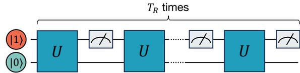
FIG. 6. **Quantum Circuit Representation for the Three-Site Ring Model.** Quantum circuit for two qubits representing the three localized states with alternating unitary  $U$  and measurements, with the initial state and target state  $|0\rangle = |01\rangle$ .
