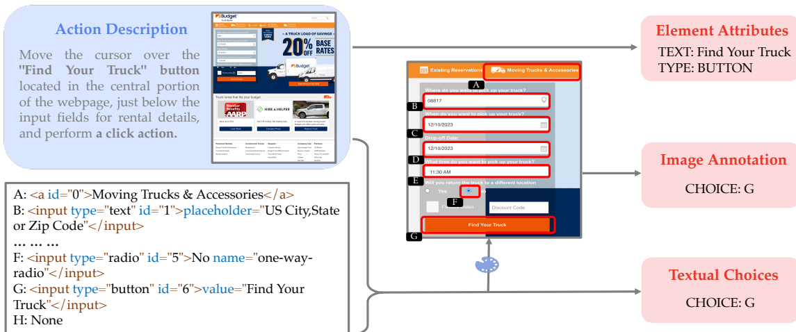
Figure 2: An example of the element grounding process for a single action during completing the given task with three different methods. In this action step, the model needs to click the "Find Your Truck" button to perform a search. For grounding with textual choices, some element candidates represented with HTML text are given, the model is required to generate the choice index of the target element. For image annotation, bounding boxes and index labels are added to the image. The model is required to generate the label on the bottom-left of the target element. For grounding with element attributes, the model needs to predict the text and type of the target element.
