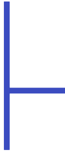
Figure 8: T shaped well with one junction and three branches of sizes 600 m (upper vertical branch), 400 m (lower left vertical branch), and 400 m (horizontal branch).
