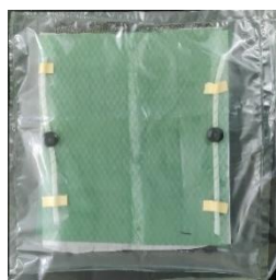
Figure 25: Vacuum bag technique
