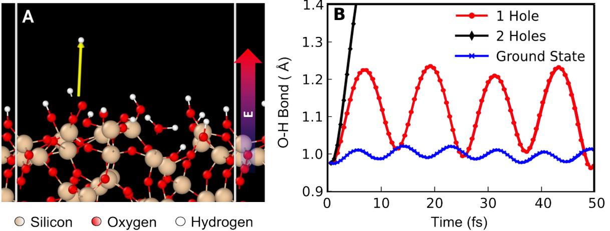
Figure 4: **Bond weakening due to the presence of surface charges** (A) Simulated silica slab representing a  $\sim 1 \text{ nm}^2$  chunk of silica in the presence of a strong DC field generated by the surface charges. The white lines depict the implemented periodic boundary conditions. (B) O-H bond dynamics with and without the presence of holes.
