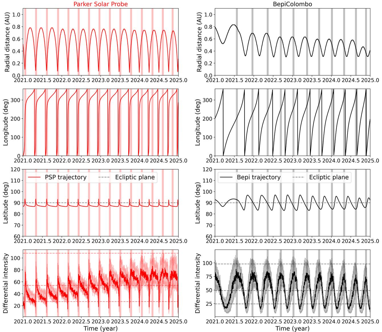
**Figure 5.** Long-term simulations of 4 MeV Jovian electrons at the position of PSP (left, in red) and BepiColombo (right, in black). Times of best magnetic connection between the spacecraft and Jupiter are also indicated by vertical shading.
