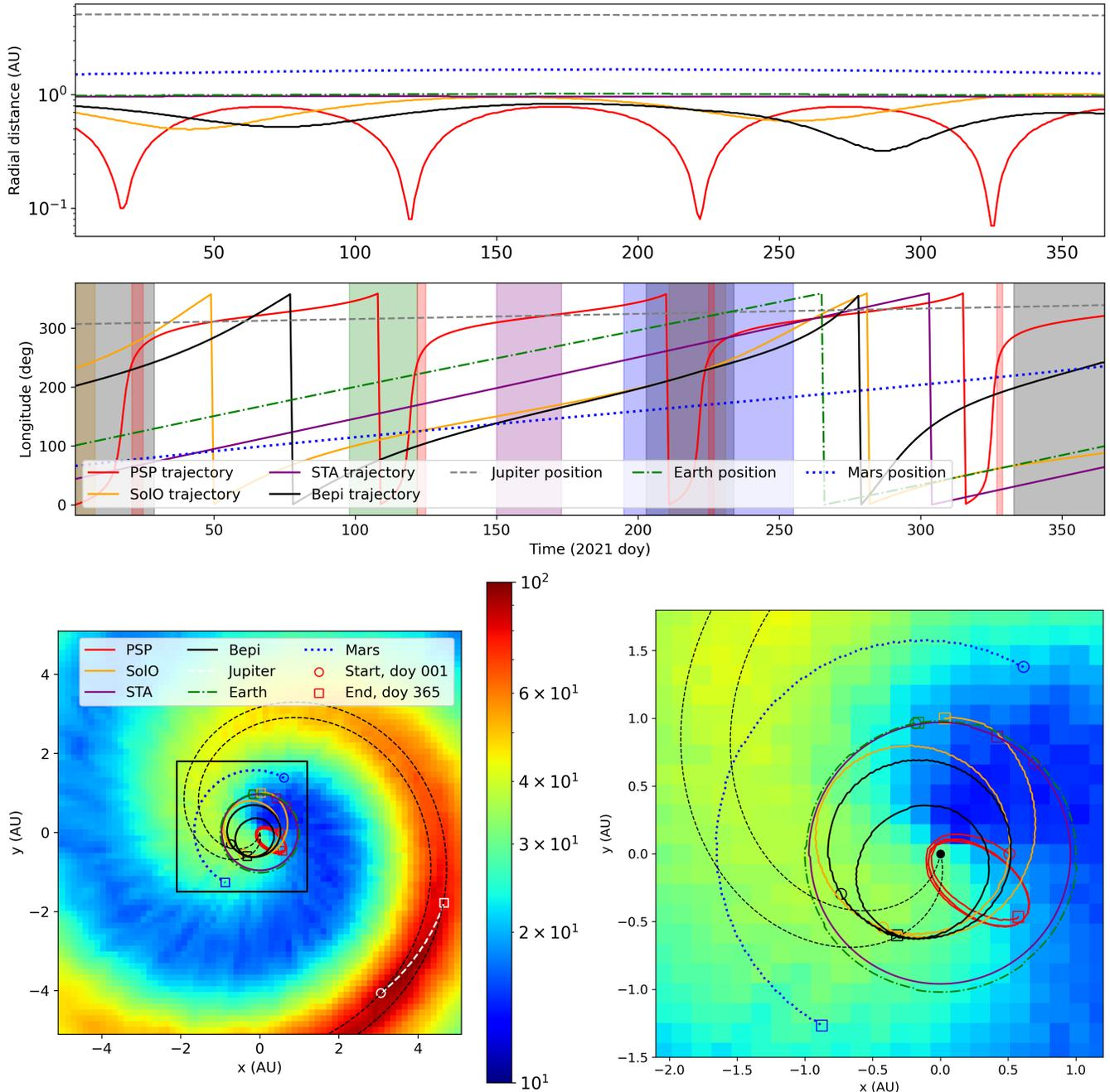
**Figure 2.** Selected spacecraft trajectories for 2021. In the bottom panels, these trajectories are overlaid onto simulation results for 4 MeV Jovian electrons with the Parker spiral field connected to Jupiter also shown. The colorbar shows the intensity, normalized to 100%, of Jovian electrons on a logarithmic scale.
