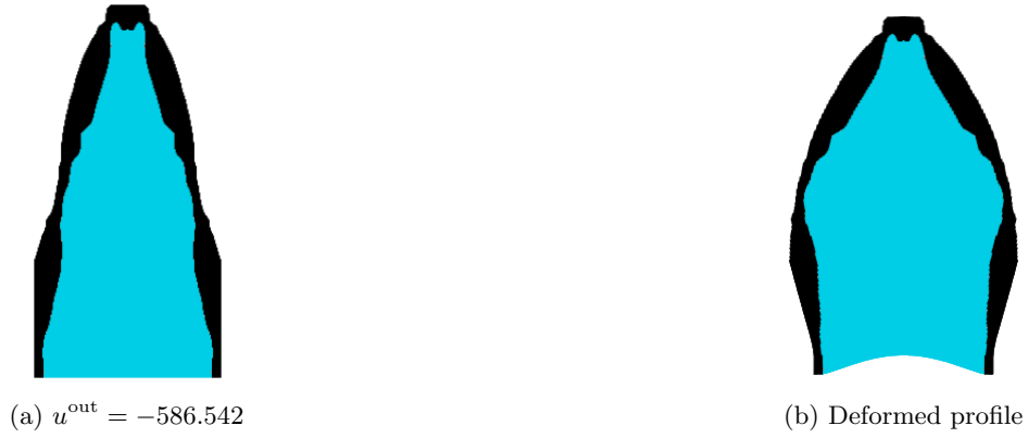
Figure 15: Optimized soft pneumatic bending actuator. (a) Optimized design and (b) Scaled deformed design
