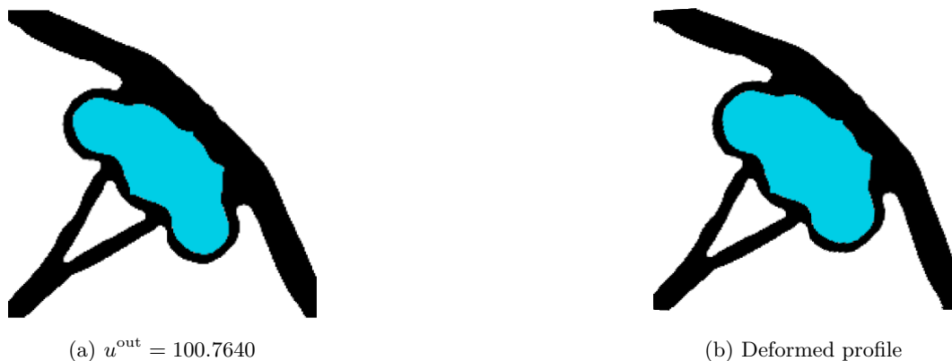
Figure 17: Optimized centrally pressurized soft pneumatic actuator. (a) Optimized design and (b) Scaled deformed design
