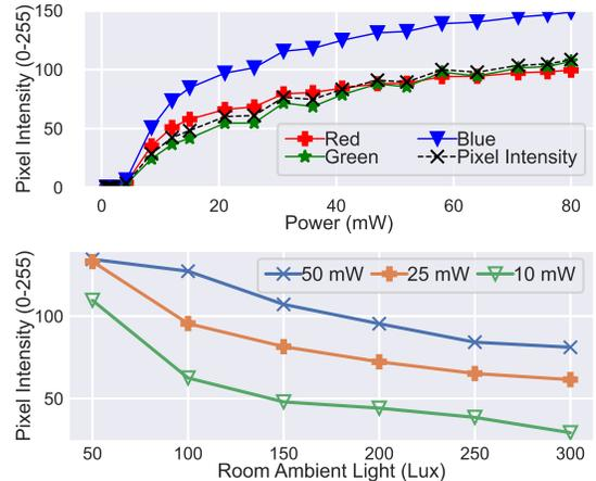
Fig. 5: 8-bit RGB pixel intensity and overall pixel intensity variation of the attack traces for  $D = 15$  cm IR pattern at increasing power (top). The impact of artificial ambient light on pixel intensity offset (bottom).
