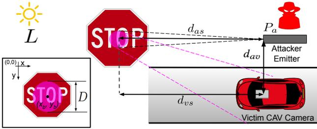
Fig. 3: Overview of parameters of ILR attack
