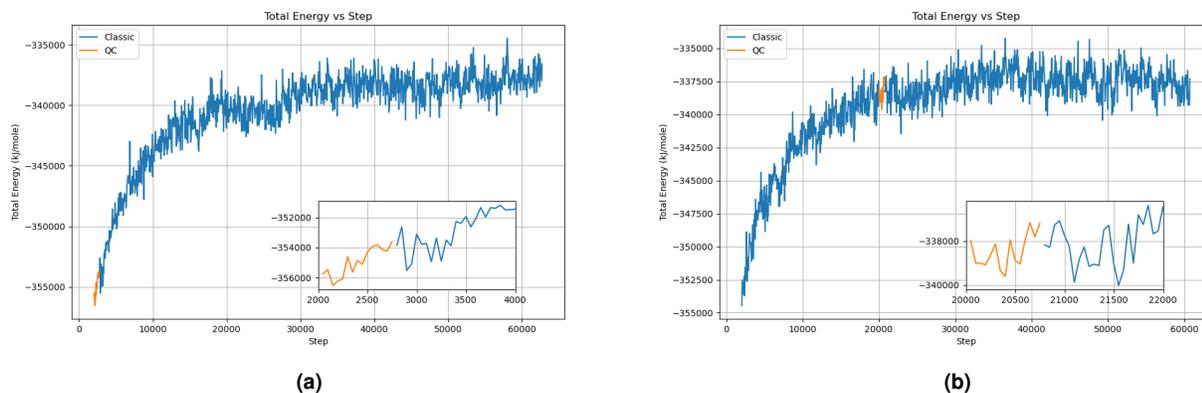
**Figure 7.** Moving key computation to the Quantum computer. Left: the simulation is started on a quantum computer, and then moved to a classical machine. Right: the simulation is started on a classical machine, moved to a quantum computer halfway, and then moved back to a classical computer.
