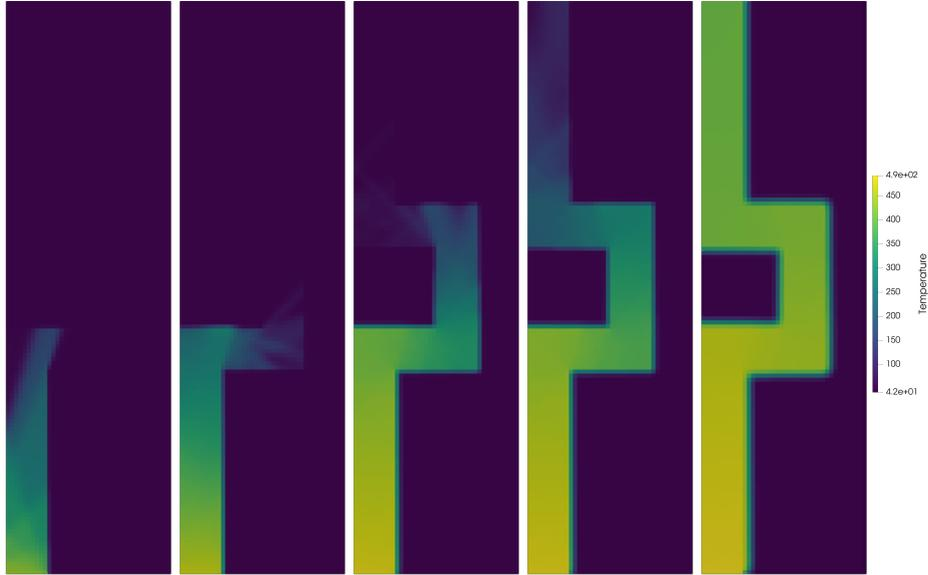
Figure 8: The evolution of the temperature at five snapshots in time. From left to right, the profiles correspond to simulation times of 0.1 sh, 1 sh, 5 sh, 10 sh, and 50 sh, respectively. Level symmetric  $S_6$  angular quadrature was used with a uniform spatial mesh of cells of size  $0.05 \text{ cm} \times 0.05 \text{ cm}$ .
