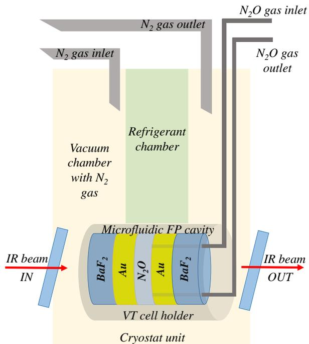
**Figure 2.** Drawing of the experimental setup for measuring ro-vibrational gas phase vibrational strong coupling of  $N_2O$  molecules.
