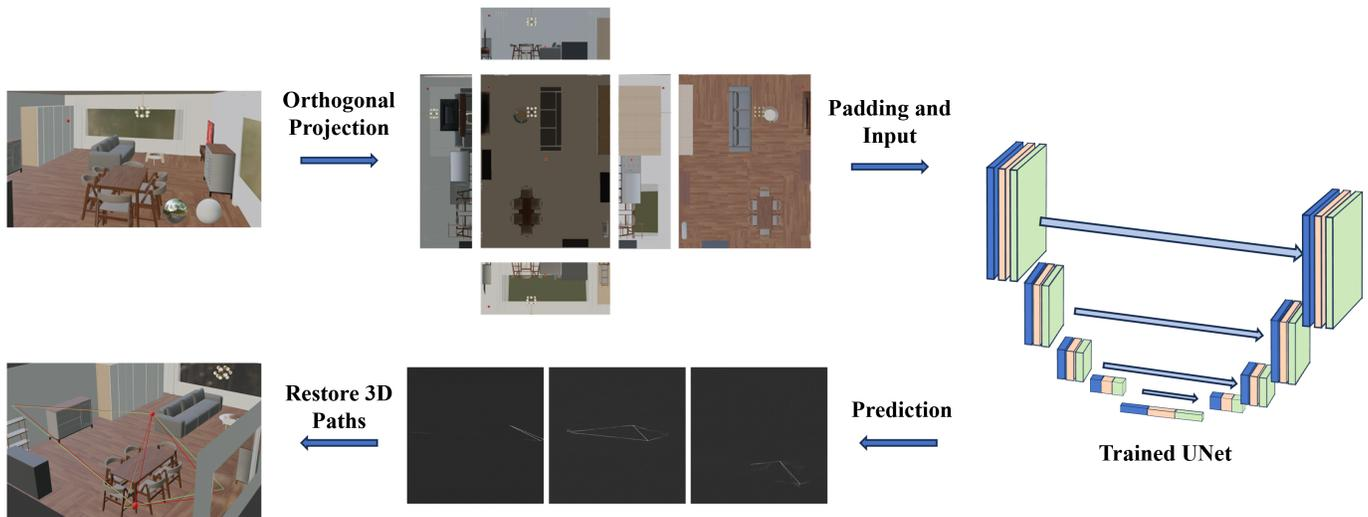
Fig. 3: Neural radio tracing to enable direct spatial-CSI prediction from images: A 3D input is projected to six views, then padded and inputted into a trained U-Net network, which predicts the 3D ray paths from three views. This network is able to implicitly learn radio propagation and interactions with objects.
