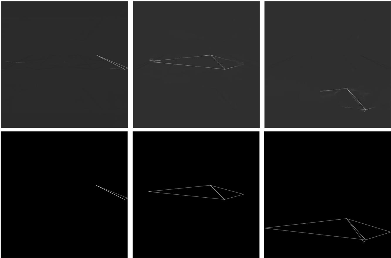
Fig. 5: Sample results of the predicted ray paths. Top: predicted results; Bottom: Ground-truth from ray tracing simulator. Background is voided for better illustration. Although blurred and missing some parts, the predicted rays are well-aligned with true spatial paths. Both training and validation data are restricted to two ray interactions.
