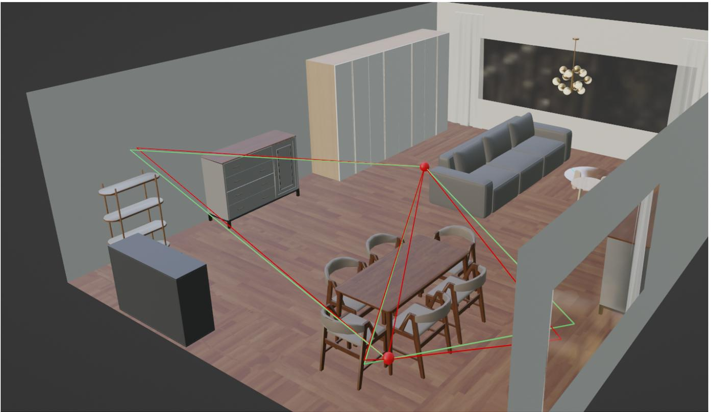
Fig. 6: Overlay the predicted paths back to the simulated 3D indoor environment. Red: ground-truth rays; Green: Predicted rays. LoS paths are fully overlapped.
