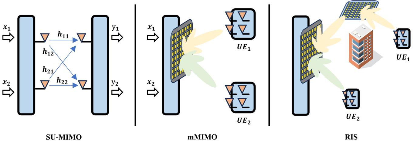
Fig. 1: Radio technologies that exploit spatial multiplexing: SU-MIMO, mMIMO, and RIS.
