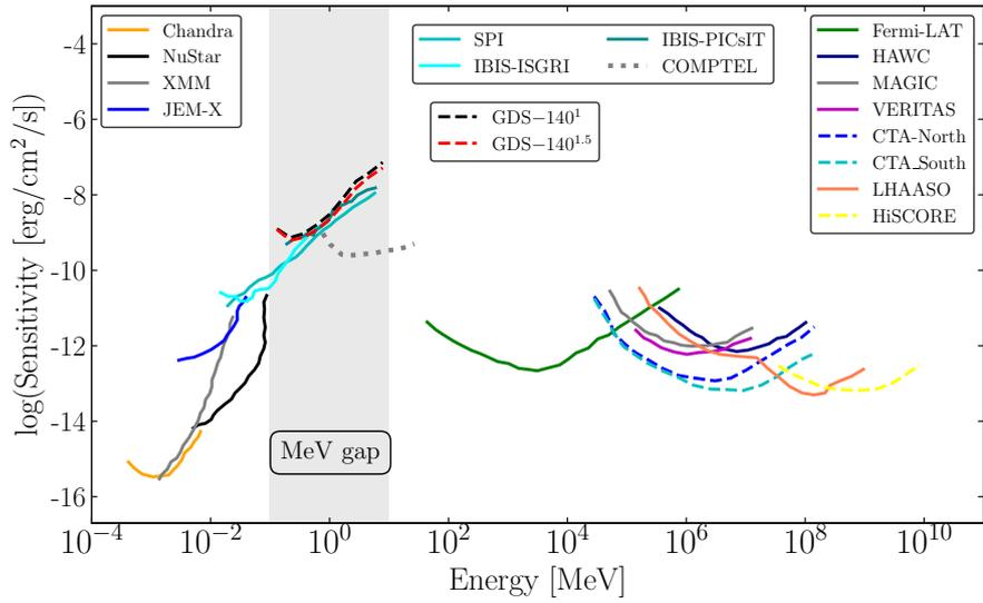
**Fig. 7** Comparison among continuum sensitivities of active instruments with **GDS-140<sup>1</sup>** and **GDS-140<sup>1.5</sup>**. Other instruments' continuum sensitivities are adopted from [Lucchetta et al \(2022b\)](#). Past/current/future missions are shown in dotted/solid/dashed lines respectively. The MeV gap is shown as a grey band.
