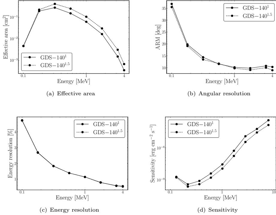
**Fig. 3** Comparison of the simulated effective area, angular resolution, energy resolution, and continuum sensitivity with crystal widths  $d = 1$  cm and  $d = 1.5$  cm for the standard **GDS-140** designs. The solid line represents **GDS-140<sup>1</sup>**, and the dashed line represents **GDS-140<sup>1.5</sup>**.
