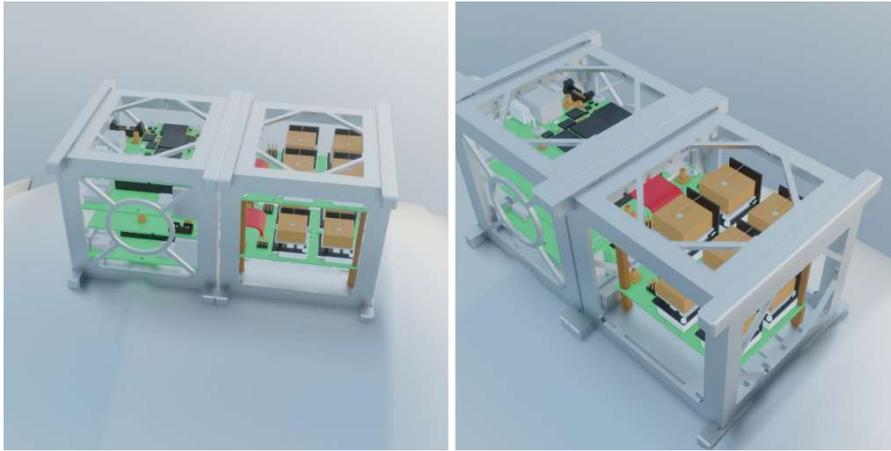
**Fig. 1** Rendered diagram of the assembled payload inside a 2U Cubesat casing with two **GDS-140** modules (shown in the right half of the 2U casing). The CZT crystals are contained within the brown “boxes”. Out of the whole 2U volume, 1U is dedicated to housing the **GDS-140** modules and another 1U is dedicated to the HV power supply unit.
