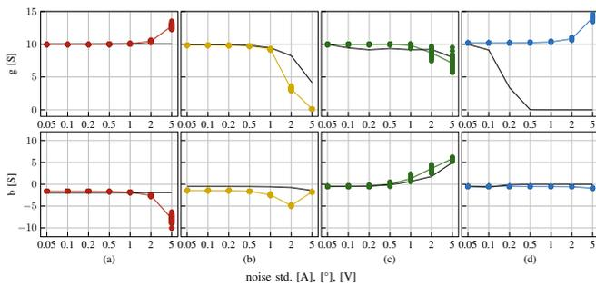
**Fig. 3:** Estimates of the conductance and susceptance of a single line using the four methods (a)-(d) with synthetic data. For each method, the points mark the estimates affected by one of the 50 realizations of the noise generated for each noise level. The line in color shows their average and the black line shows the predicted bias. In case (d) the black line is a lower bound on the bias.
