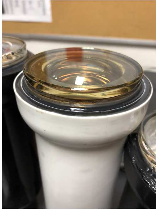
Figure 11: The photocathode of a Madison PMT exposed to the environment. The tube was glued into the plastic insert (white) with a resin potting compound (black). This created a waterproof seal between the glass and the plastic.
