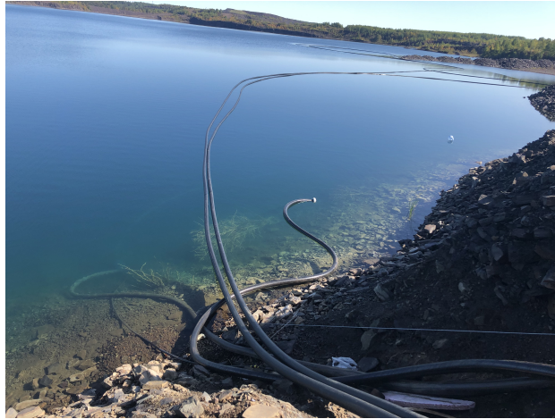
Figure 9: The completed inflow and outflow water pipes for the detector. The third, shorter pipe is the water intake from the mine pit, which was used for filling the detector during deployment.
