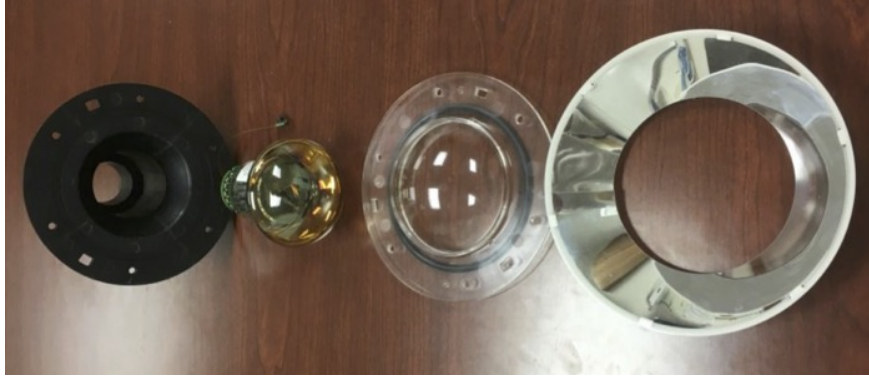
Figure 12: Disassembled Nikhef PMT. From the left: plastic insert, the PMT itself with its HV base attached, the waterproof cover complete with its O-ring, and finally the plastic light reflector.
