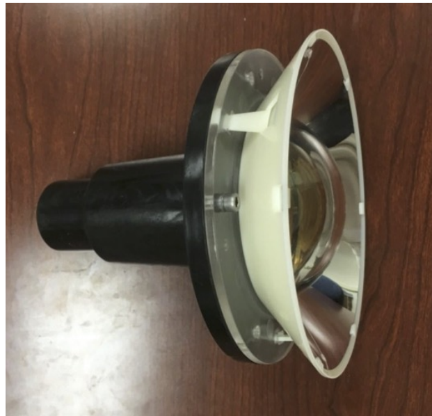
Figure 13: Assembled Nikhef PMT, ready to be glued onto a plane.
