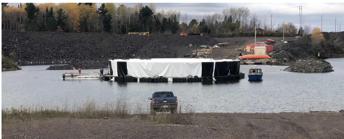
Figure 16: The exterior of the detector after completion. The liner can be seen supporting the detector and the floating dock forms a perimeter around the detector. Two boats tow and steer the detector during deployment. The scale of the detector is visible.
