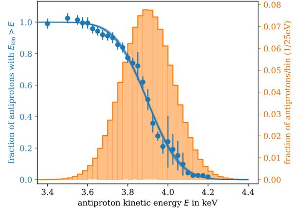
**Figure 9:** The energy distribution of decelerated antiprotons. The data and fitted CDF of a normal distribution are shown in blue, and the probability density function corresponding to the fit in orange. The mean energy is  $\mu = (3898 \pm 3) \text{ eV}$  and the standard deviation  $\sigma = 127 \pm 4 \text{ eV}$ . 88% of decelerated antiprotons are within  $\pm 200 \text{ eV}$  of the mean energy, which is the estimated energy acceptance for trapping.
