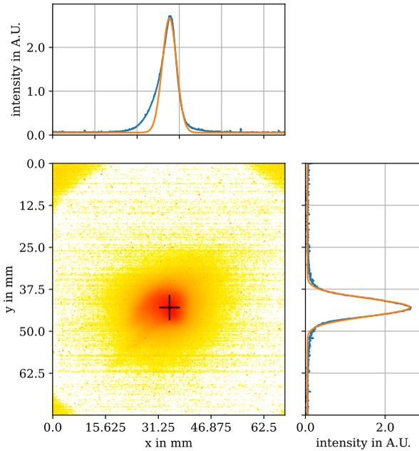
**Figure 8:** Beam profile after optimizing the LV einzel lenses for deceleration to 4 keV and focus on the BTV. Fitting a Gaussian to the centre peak yields  $\sigma_{\text{horiz}} = 3.0 \text{ mm}$ ,  $\sigma_{\text{vert}} = 3.8 \text{ mm}$ . Yellow indicates a lower and red a higher intensity.
