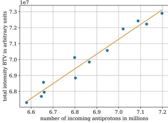
**Figure 7:** The bunch intensity of antiprotons determined by the ELENA detectors is proportional to total intensity on the BTV. The transmission to the BTV is 100% when not decelerating the antiprotons. This allows to make a calibration to determine the transmission through the pulsed drift tube while decelerating.
