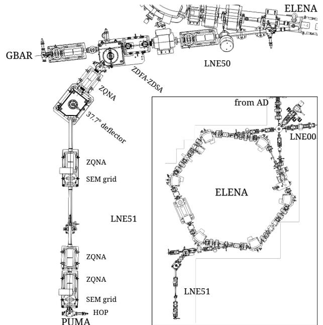
**Figure 1:** Schematic view of LNE51 transfer line to PUMA. Antiprotons are ejected from ELENA into LNE50, from which LNE51 branches off. The insert shows the position of LNE51 relative to ELENA and LNE00.
