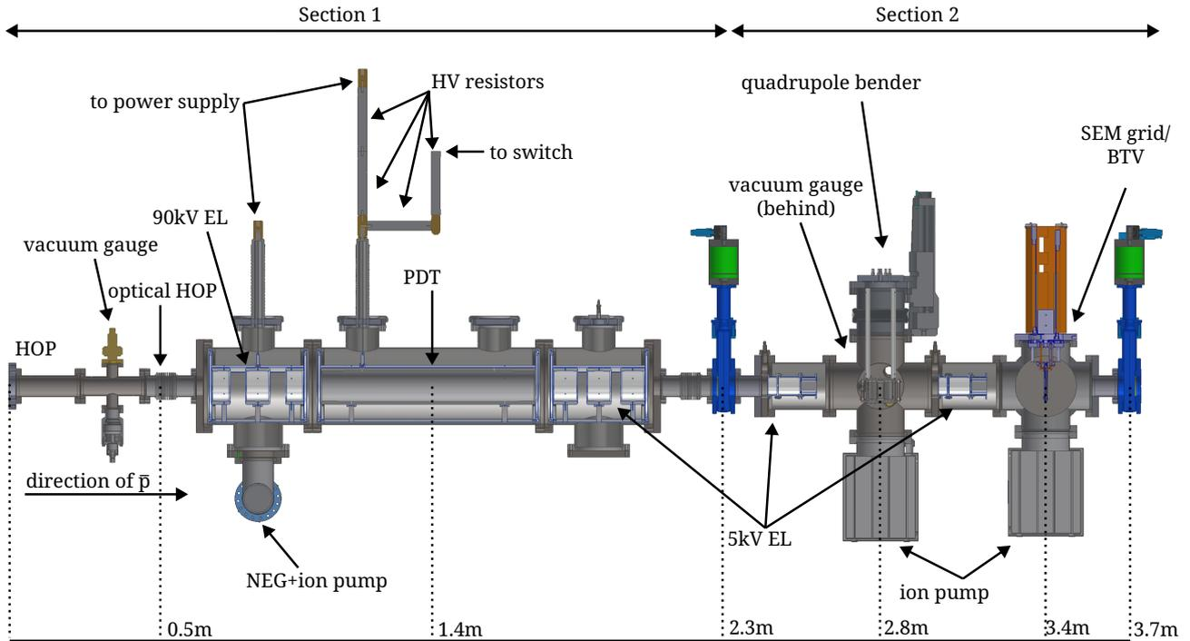
**Figure 2:** Half-section view of the beamline without the supports. The antiprotons traverse the beamline from left to right. Ions from the offline source enter the beamline at the quadrupole bender in the direction into the page and are deflected to the right. The gate valves separating the sections are depicted in blue.
