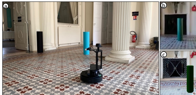
Fig. 1. We perform Multi-Object Navigation [41], i.e. the sequential visual search of multiple object in a given order, and are the first to do this in real physical environments (a) characterized by a large sim2real gap. This is illustrated by two first-person views (b), real and (c), simulation. We propose a hybrid method combining classical mapping and deep learning, and compare to the SOTA methods on this task using end-to-end RL training and auxiliary losses [28].
