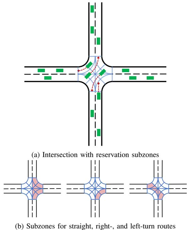
Fig. 1: **Geometry of our studied intersection.** Our algorithms are applicable to junctions in general, e.g. merging, as the exact geometry is encoded by the start and end positions of subzones along vehicle routes,  $x_{z,r}$ .
