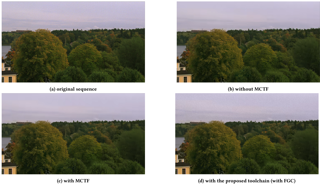
Figure 5: Comparison of the representative (cropped) frame of IntoTree test sequence encoded at 0.25 Mbps.
