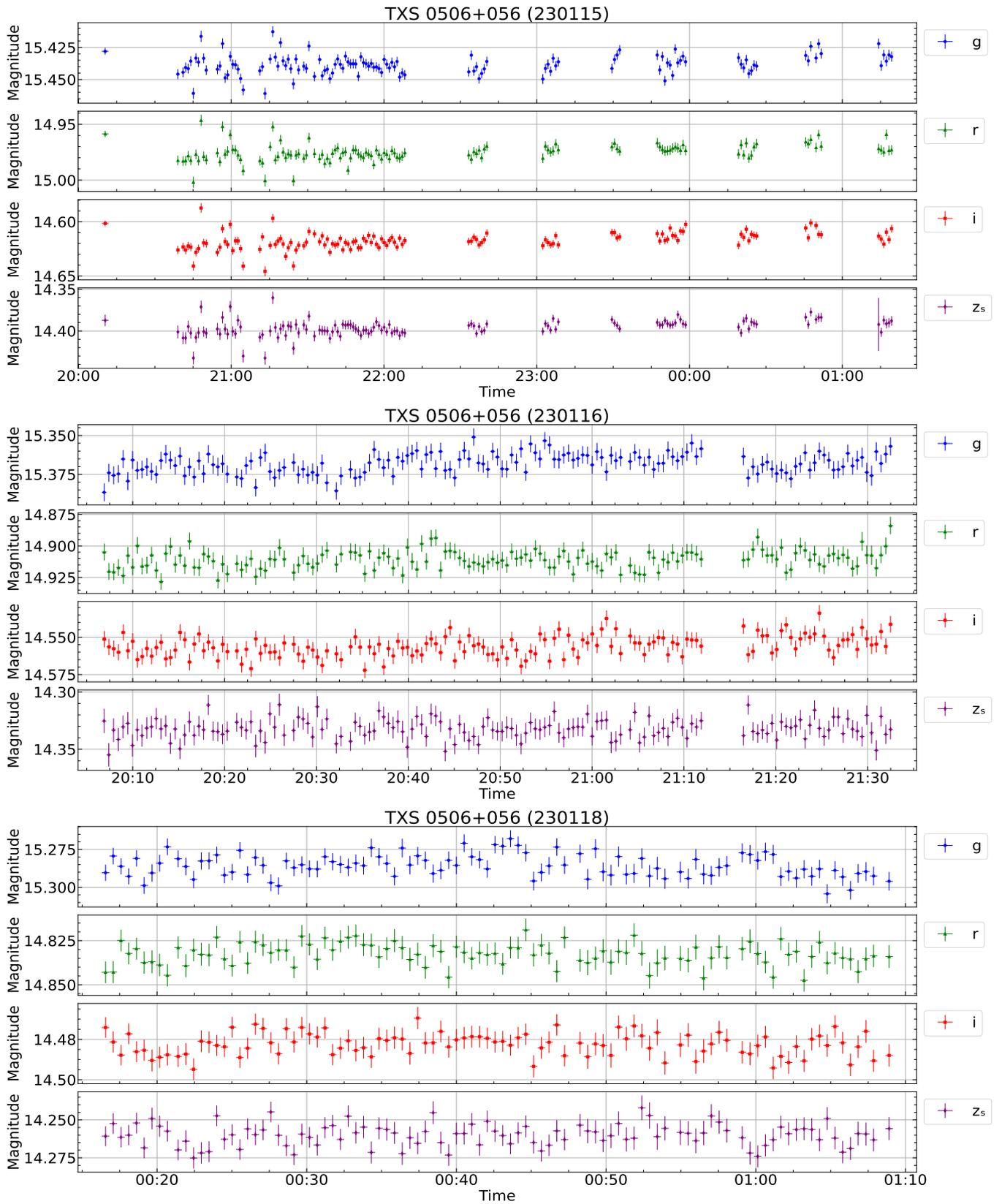
**Figure B1.** Light curves of TXS 0506+056 on the nights of 2023 January 15, 2023 January 16, and 2023 January 18. The panels of each of the three plots correspond to *g*, *r*, *i*, and  $z_s$  filters, from top to bottom.
