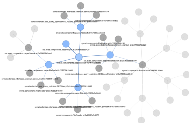
Figure 5: We illustrate the hierarchical computational graph for the Paper expression. Each node represents an instance of an expression with distinct properties and behaviors, such as file sourcing, generative process, tool utilization, or transformation operation. The edges denote the reference relationships between expressions and indicate the flow of information. The blue highlighted nodes mark the main sequence nodes of expressions utilized to create parts of the paper draft, such as Method section, RelatedWork section, Abstract section, and so on. Each generative node is used for evaluating the VERTEX score. None-generative nodes such as search engine results are not evaluated, and we assume to obtain ground-truth values.
