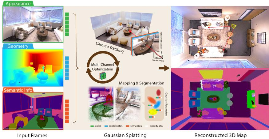
**Fig. 1:** The illustration of the proposed SGS-SLAM. It employs 2D inputs encompassing appearance, geometry, and semantic information, leveraging Gaussian Splatting and differentiable rendering for multi-channel parameter optimization. During the mapping process, SGS-SLAM maps the 2D semantic prior to the 3D scene, jointly optimizing it via the mapping loss for accurate 3D segmentation outcomes.
