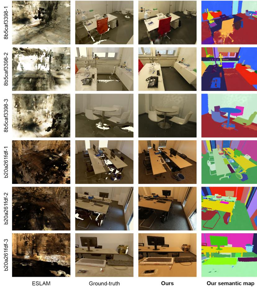
**Fig. 9:** The visualization of novel view rendering between the baseline and our method using the ScanNet++ dataset [43]. The ground-truth novel views are captured from meshes. SGS-SLAM demonstrates superior rendering quality, while ESLAM [15] suffers from significant tracking errors and fails to reconstruct the map. In addition, our method also offers accurate instance-level segmentation outcomes.
