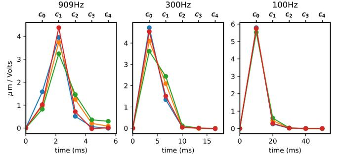
**Fig. 1.** Open loop response of the piezo control chain. This corresponds to the response of the piezo in micrometers per volt, as a function of time (bottom axis), when submitted to an impulse command. Equivalently, this also gives the values of the coefficients of the fifth order model used in Equation 20 (top axis). Each colour represents a distinct actuator.
