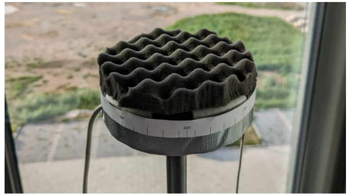
Fig. 4: UCA Microphone Array with a windscreen for outdoor usage. Details of the employed algorithms can be found in [43]
