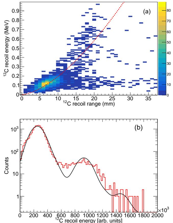
FIG. 4. Selection of ( $^{13}\text{N}, p_{0,1}$ ) events. Top: Experimental data of  $^{12}\text{C}$  recoil range in TPC versus energy. The expected result from TRIM [11] is overlaid as a dotted red line. Bottom: Proton energy spectrum from these data obtained from the  $^{12}\text{C}$  recoil (red histogram). The expected yield using previously-obtained branching ratios [12] is overlaid as a black solid line after being convoluted with a Gaussian profile to best replicate the data.
