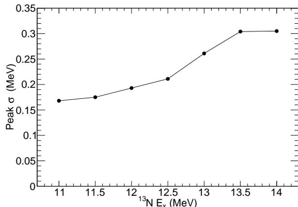
FIG. 12. Variation of experimental resolution from a GEANT4 simulation of infinitely narrow states decaying via  $^9\text{B}(\text{g.s.}) + \alpha$  as a function of excitation energy. The statistical error bars are not shown as the error for each point is dominated by systematic errors via the stopping power uncertainties for  $\alpha$ -particles and may be as large as 0.1 MeV (towards larger peak  $\sigma$  values).
