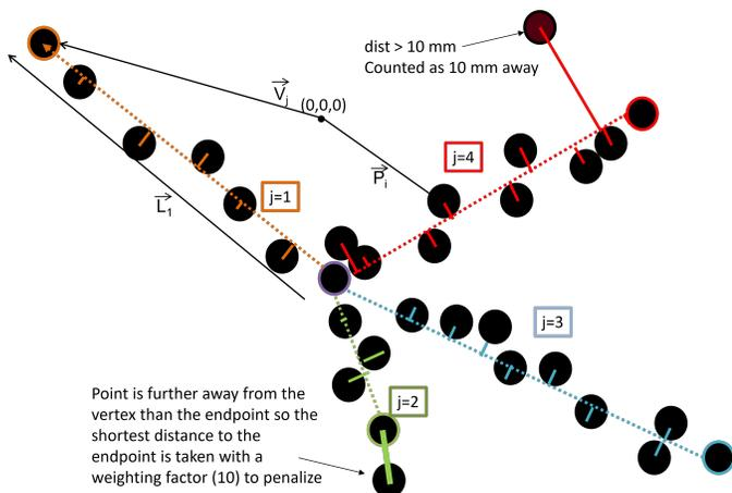
FIG. 5. Schematic showing the basis of the RANSChiSM fit by selection of five points to parameterize the four-track fit. Any points in the pointcloud more than 10 mm from the nearest track line are counted as if they are 10 mm away to reduce the influence of outliers.
