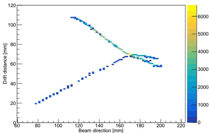
FIG. 10. An example  $\alpha_0$  ( $^9\text{B}(\text{g.s.}) + \alpha$ ) event where the energy deposition as a function of distance in the TPC is shown projected in 2D. The track going downwards can be identified as the proton by its lower energy deposition. Also shown in [5].
