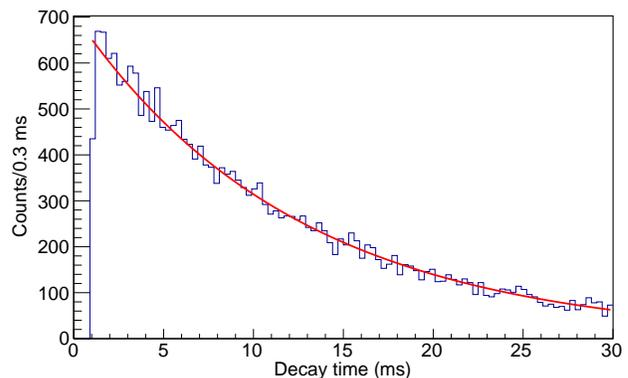
FIG. 3. Decay time between the implant of  $^{13}\text{O}$  and decay overlaid with a background free exponential fit yielding a value of  $t_{1/2}=8.55\pm 0.09$  (stat.) ms compared to the adopted value of  $8.58\pm 0.05$  ms [10].  $\chi^2 = 1.26$  from log-likelihood minimization.
