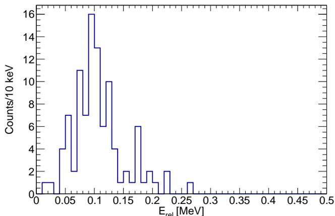
FIG. 6. Relative energy spectrum for pairs of  $\alpha$ -particles (taking the smallest relative energy) showing the  ${}^8\text{Be}(\text{g.s.})$  energy of 92 keV is well-reproduced in our data.
