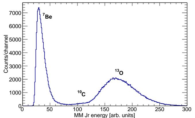
FIG. 2. Energy deposition (dE) within the Micromegas Jr detector to differentiate the beam species. The contaminants to the  $^{13}\text{O}$  were dominated by  $^7\text{Be}$  and they total  $\approx 28\%$  of the total beam intensity of 5 pps.
