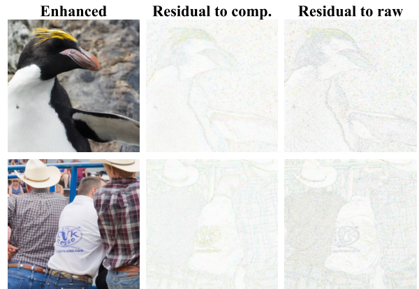
Figure 4. Residual comparisons between enhanced images [44] and their compressed/raw counterparts. These visualizations reveal a stronger resemblance of the enhanced images to their compressed counterparts, as indicated by the weaker residual.
