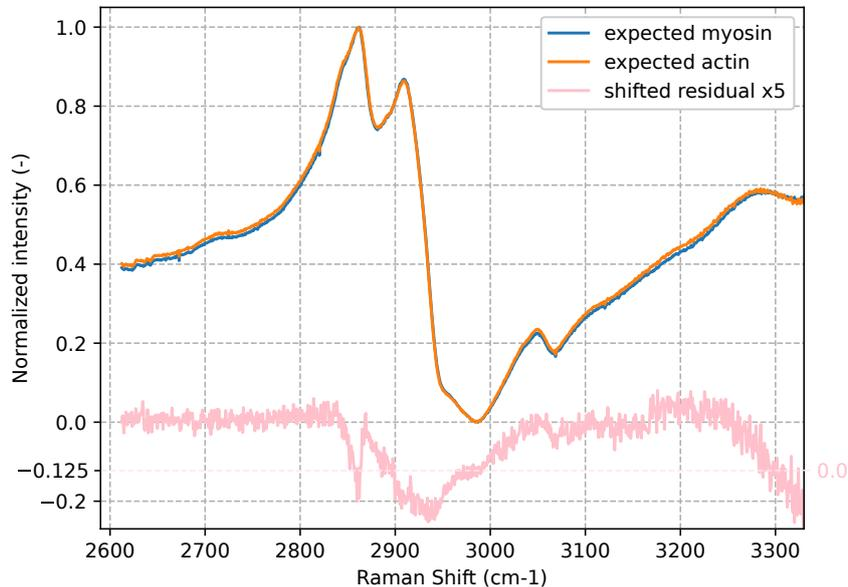
*Figure 3: Average M-CARS spectra from locations highlighted as myosin (blue) or actin (orange) from the SHG image in Figure 2 (b). For sake of clarity, their differences are presented shifted by -0.025, and multiplied by 5 (pink).*
