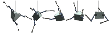
Fig. 4: SpaceHopper reorienting itself to the upright orientation, which is displayed as a black line.
